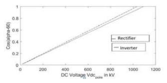
**Fig. 2** : Theoretical relation between  $Cos (alpha - 60^{\circ})$  and  $Vdc_{note}$  during normal power flow operation
