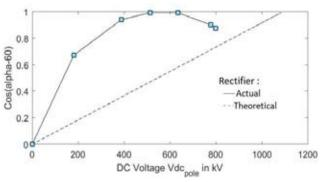
**Fig. 5** : Theoretical and actual relation between *Cos* (*alpha* – 60°) and  $Vdc_{pole}$  for rectifier during OLT
