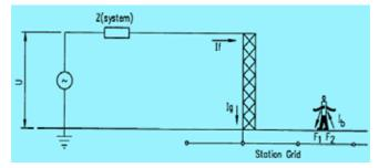
Fig. 5 : Different Resistances of Circuit for Step Voltage
