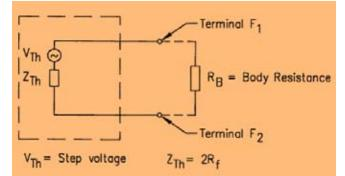
Fig. 6 : Thevenin Equivalent of Circuit of figure 5
