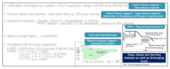
These parameters are now the "Key reliability indices" as well as "Emerging tools" for further analysis, monitoring & considerations of system strength as well as operational aspects to enhance the grid strength by improving steady as well as dynamic performance of the grid.
