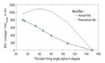
Fig. 4 : Theoretical and actualrelation between Vdc<sub>pole</sub> and alpha for rectifier during OLT
