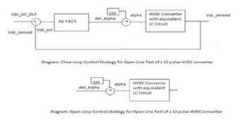
Fig. 6 : Closed and Open Loop control strategy for Open Line Test of a rectifier
