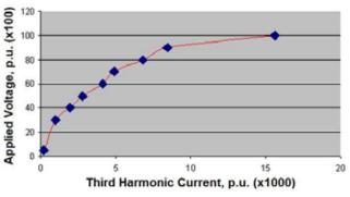
Fig. 5 : Variation of third harmonic component of leakage current with respect to applied voltage
