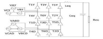
Fig. 11 : Schematic diagram of 12 pulse bridge ac to dc converter in open loop condition
