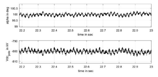
Fig. 19 : Closed loop simulation of (-vepole) of Station 2 with circuit configuration 3(a). DC Voltage command = -800 kV
