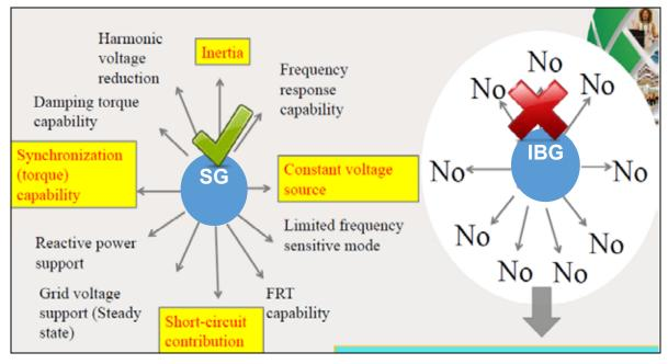
Fig. 3 : Characteristics Difference between SG and IBG
