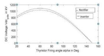
**Fig. 3** : Theoretical relation between *Vdc*<sub>pole</sub> and *alpha* during normal power flow operation
