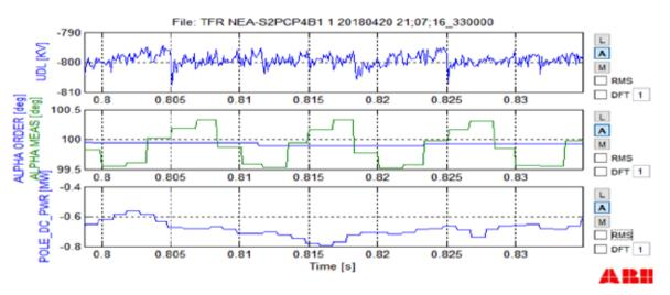
**Fig. 20** : Negative pole of Station 2 with circuit configuration 3(a). DC Voltage command = 800 kV without considering the sign.
