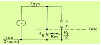
Fig. 3 : Different Resistances of Circuit for Touch Voltage
