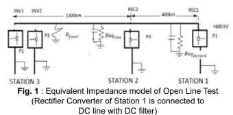
Equivalent circuit model has been taken from the configuration of ±800kV NEA-Agra multi-terminal HVDC system.
