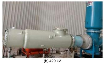
Fig. 3 : Experimental Set-up for Measurement of Leakage Current
